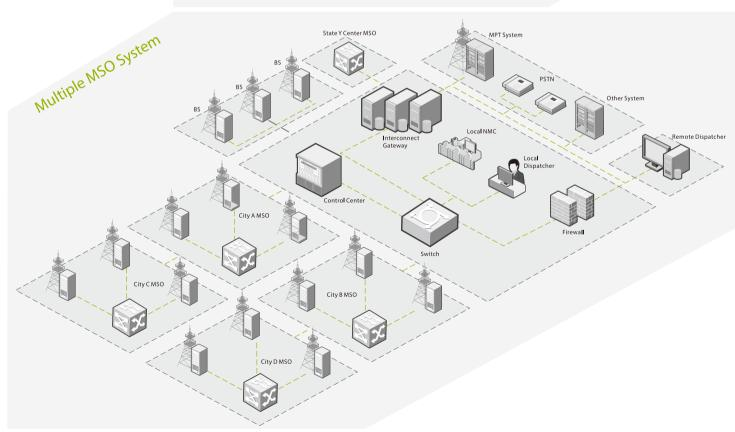
As the core of Hytera DMR Trunking Pro, MSO comprises a wide array of subsystems to enrich the application functions, such as Network Management System (NMS), Dispatching System and Digital Voice Recording System (DVRS).
